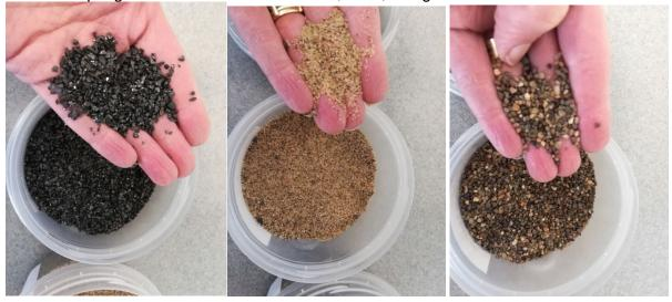
Once in the filter chamber, the water flows down through the filter material; anthracite coal, sand, gravel and ceramic filter screens.
