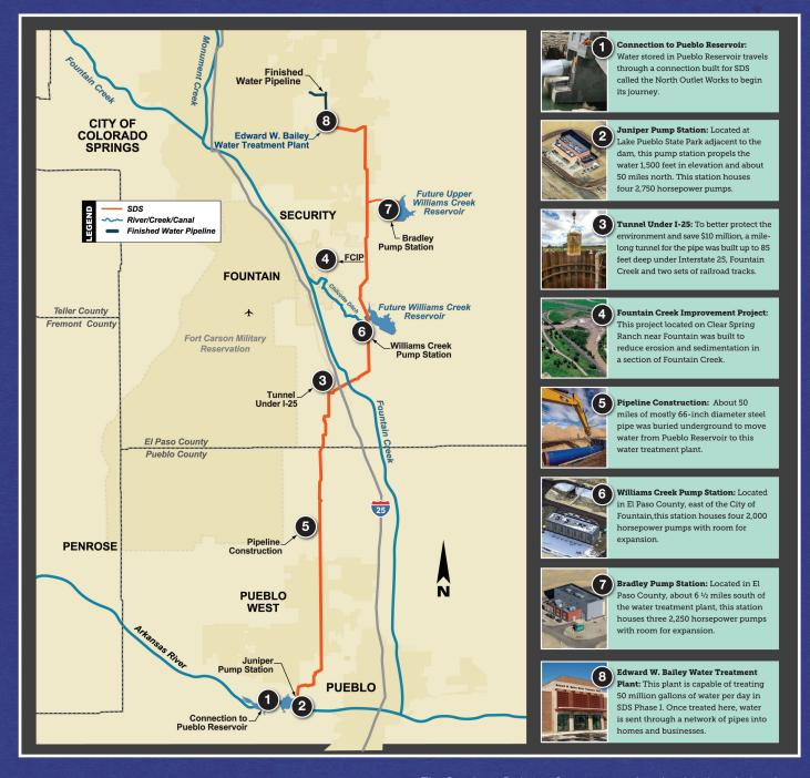
The Southern Delivery System, completed in 2016, includes about 50 miles of raw and finished water pipeline, three pump stations and the Edward W. Bailey Water Treatment Plant.
