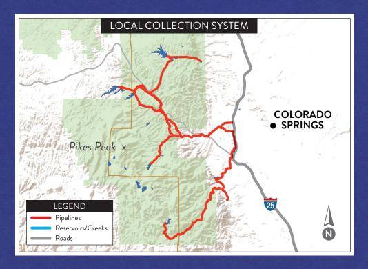
Our local system, including Northfield, North Slope and the South Slope systems. Northfield is fed mainly by our trans-mountain systems and delivers water to Pine Valley and McCullough treatment plants. South Slope and North Slope deliver water to the Mesa Water Treatment Plant.
