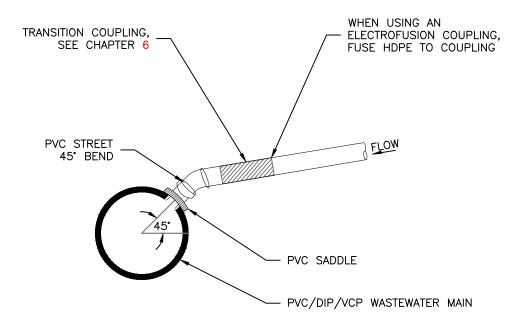
HDPE SERVICE LINE TO PVC/DIP/VCP WASTEWATER MAIN
