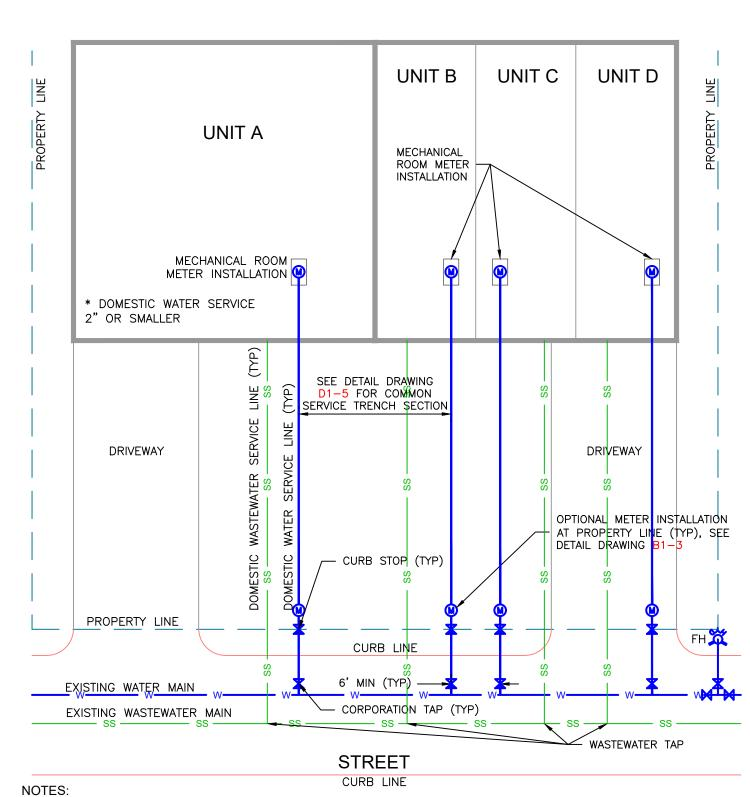
1. THIS DETAIL DRAWING APPLIES TO A SINGLE PLATTED LOT WITH MULTIPLE DWELLING UNITS, WHERE EACH UNIT IS CONNECTED AND METERED SEPARATELY. IF THE PROPERTY IS SUBDIVIDED, INDIVIDUAL SERVICE LINES SHOULD BE INCLUDED ON THE INDIVIDUALLY PLATTED LOT. IN THE ALTERNATIVE A PRIVATE EASEMENT SHOULD BE PROVIDED TO ACCOMMODATE WATER SERVICE LINES THAT MAY CROSS ANOTHER PLATTED LOT.
