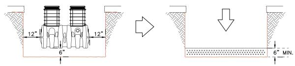
EXCAVATE HOLE AT LEAST 12" LARGER THAN INTERCEPTOR ON ALL SIDES AND 6" DEEPER THAN TANK BOTTOM.
