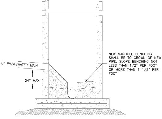
1. SEE DETAIL DRAWING C3-1 FOR MANHOLE REQUIREMENTS.
