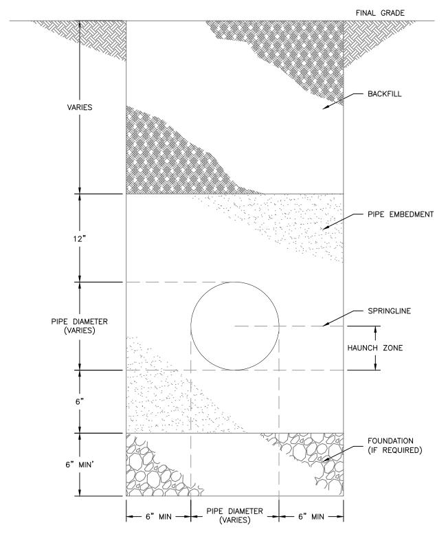
1. TRENCH BACKFILL SHALL CONFORM TO THE SPECIFICATIONS OF THE AUTHORITY HAVING JURISDICTION AND ASTM D2321.
