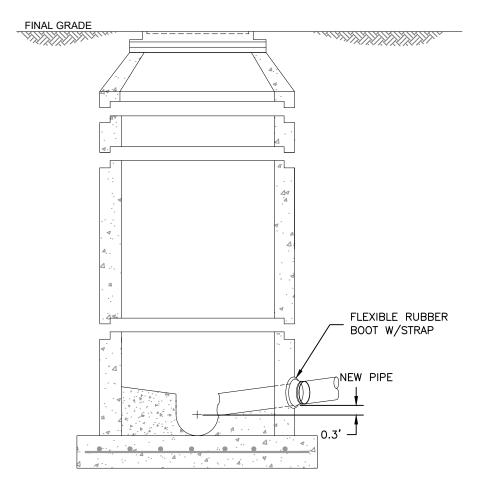
1. SEE DETAIL DRAWING C3-1 FOR MANHOLE REQUIREMENTS.
