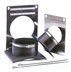
**General:** Saddle Taps may be an EPDM rubber gasket with locating/centering ring with corrosion resistant Series 300 austenitic stainless steel apron fastened with 300 series stainless steel bands, full 9/16" width band with a cadium plated carbon steel 5/16" shouldered hex head slotted screw.
