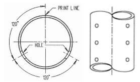
Figure 8-1: Perforated Pipe Hole Configuration
