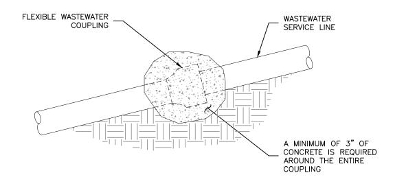
1. IF THE FLEXIBLE COUPLING IS "SHIELDED" VARIETY PER CHAPTER 4, NO CONCRETE IS REQUIRED AROUND THE COUPLING.
