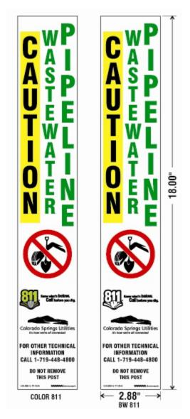
**General:** Line markers are to be installed with Colorado Springs Utilities decal and telephone number.
