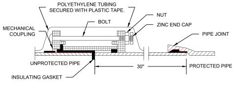
INSULATED MECHANICAL COUPLING
