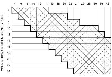
INDICATES THAT A CONCRETE THRUST REACTION BLOCK IS REQUIRED
