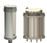
Large orifice sealing shall be affected by the flat face of the control float seating against a nitrile/EPDM rubber 'O' Ring housed in a dovetail groove circumferentially surrounding the large orifice. Discharge of pressurized air shall be controlled by the seating and unseating of a small orifice on a natural/EPDM rubber seal affixed to the control float.
