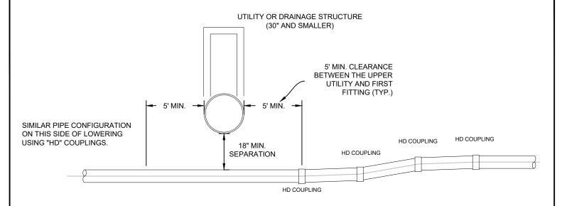
HIGH DEFLECTION COUPLING (4"-12") 4° DEFL. (i.e. MAX. 2° IN AND OUT OF COUPLING) (REFERENCE DETAIL DRAWING A4-1)
