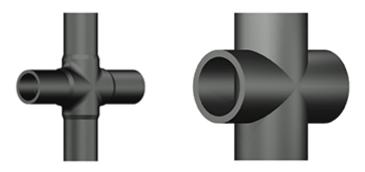
Crosses are rarely used and must come with attached fitting ends to fit into a valve or reducer. Care must be taken when placing a cross in the trench to avoid stress fractures in the center of the cross.
