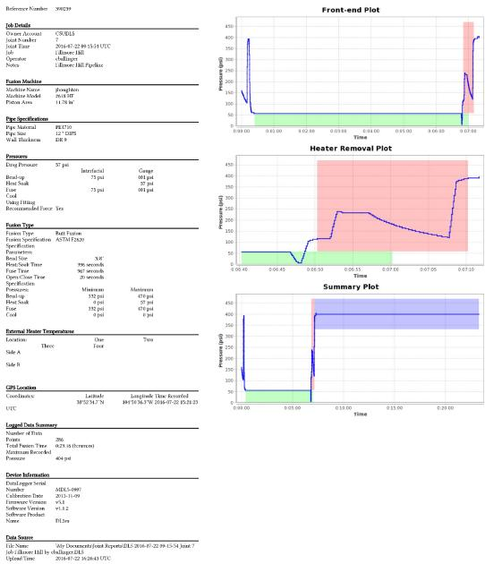
Figure 6-1: Example of a Heat Fusion Joint Record (typical output for a McElroy Data Logger)
