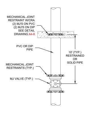
IN LINE VALVE INSTALLATION
