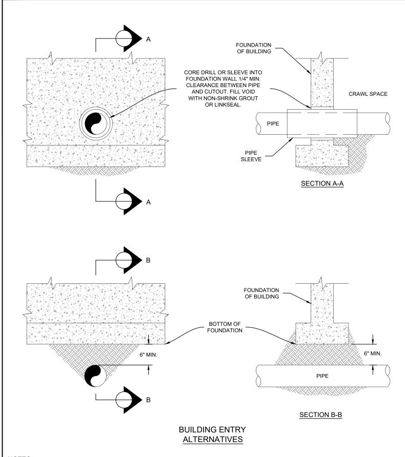
1. WHERE COMPACTION CANNOT BE ACHIEVED UNDER THE WATER MAIN FLOWFILL SHALL BE USED.
