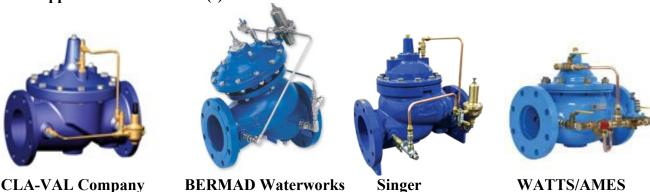
**General:** The valves shall be capable of maintaining a constant downstream pressure regardless of varying inlet pressures. When the downstream pressure exceeds the pressure setting of the control pilot, the main valve and pilot valve shall close drip-tight.
