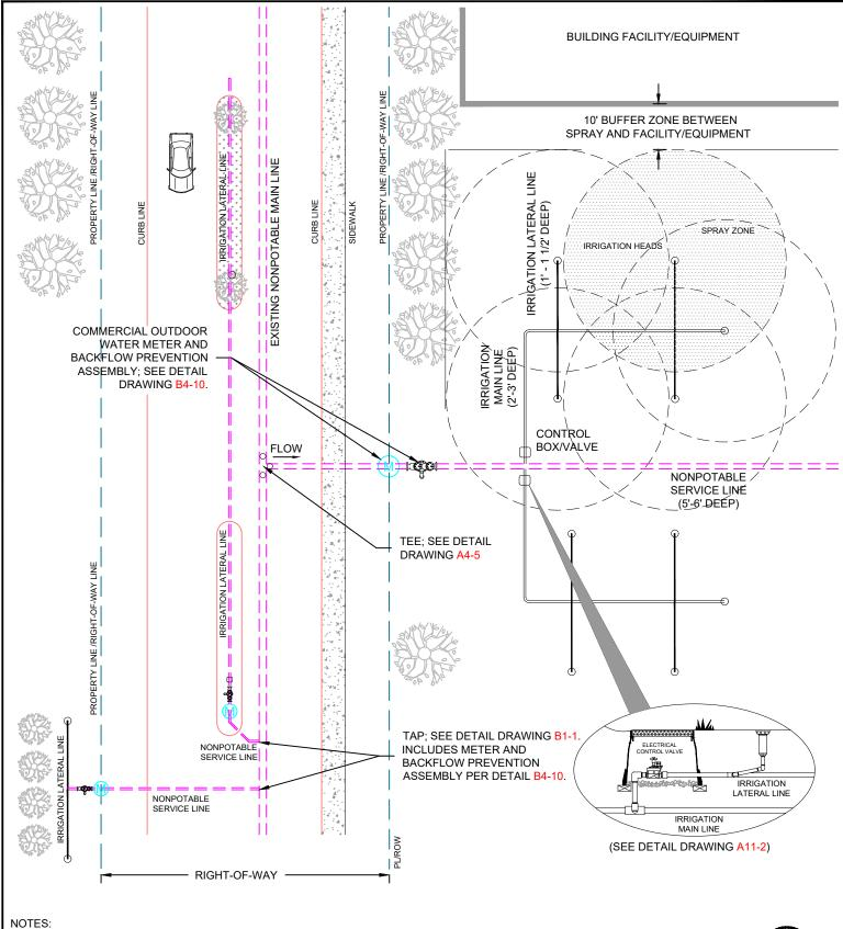
NONPOTABLE SERVICE LINES, THAT CROSS OVER A POTABLE WATER LINE OR SERVICE SHALL BE SLEEVED APPROXIMATELY 5 FEET EACH SIDE OF THE CENTER OF THE POTABLE WATER LINE.
