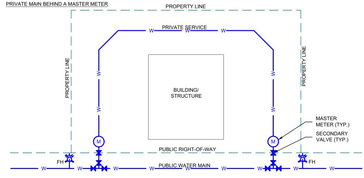
1. PRIVATE WATER MAINS BEHIND A MASTER METER ARE ALLOWED BUT NOT RECOMMENDED DUE TO FIRE FLOW AND BACKFLOW PREVENTION WATER METER REQUIREMENTS AND OWNERSHIP RESPONSIBILITIES.
