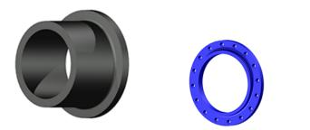
Flange adapters shall be made with sufficient through-bore length to be clamped in a butt fusion-joining machine without the use of a stub-end holder. The sealing surface of the flange adapter shall be machined with a series of small v-shaped grooves (serration) to promote gasket-less sealing, or restrain the gasket against blowout. A Beveled Flange Adaptor is for use with Butterfly Valves.
