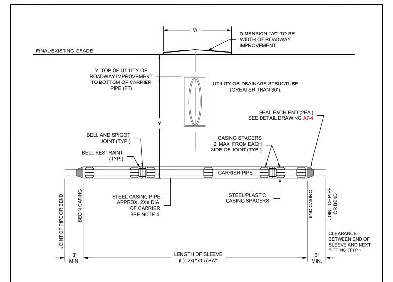
AN ADDITIONAL CASING SPACER SHALL BE CENTERED ON THE PIPE WHEN 18' TO 20' LONG PIPE JOINTS ARE USED. (TYP.)
