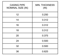
CASING PIPE MINIMUM SIZES AND THICKNESSES ARE BASED ON E80 LOADING. VARIANCES TO THESE MINIMUMS MAY BE ALLOWED WITH SUPPORTING CALCULATIONS FROM THE DESIGN ENGINEER
