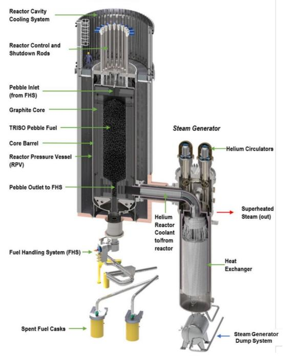
Figure 5 Rendering Showing the Xe-100 Reactor System and SGS Major Components.
