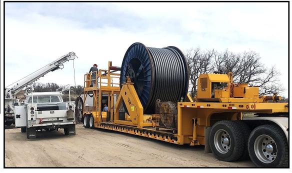
Underground Reel on Custom Trailer for Cable Pulling
